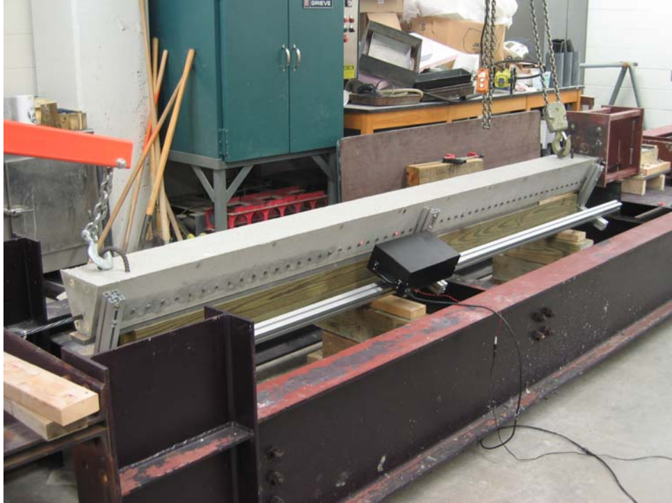
Figure A4. Testing the prototype laser-speckle strain-measurement device on a prestressed concrete member. In this experiment, the data were compared with data collected using de-mountable mechanical (DEMEC) gage points.
